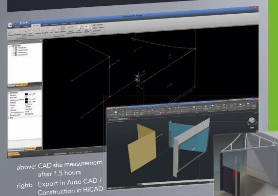
The easy SOLUTION for this measurement was the use of the Flexijet 3D system, which measured and drew the object at the same time. Measurement service provider Konrad Schwegler collected all relevant dimensions within 1.5 hours on site.
